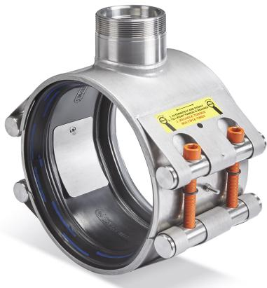
PEWOREP PN 10 NOT TENSION-PROOF with Connection piece with 2" Internal thread EPDM Sealing -30°C up to +80°C in A4 (316/1.4571) Quality Ø min./max. 210-223 mm Width 142 mm 2 Closure Country of origin: EU TARIC: 73072980
