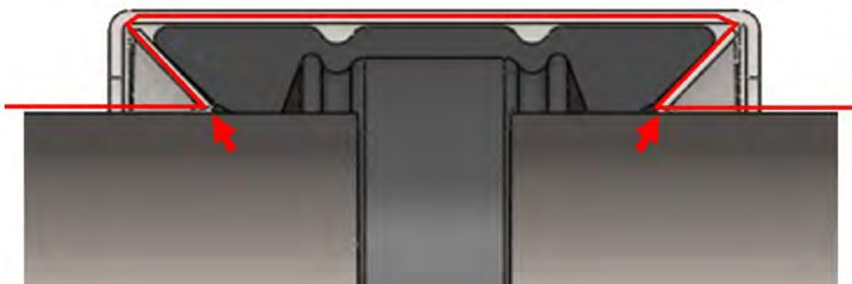
PEWOCOUPING pipe couplings of the series PEWOGRIPI ensure electrical bridging from pipe to pipe as a result of the metallic anchoring mechanism.
